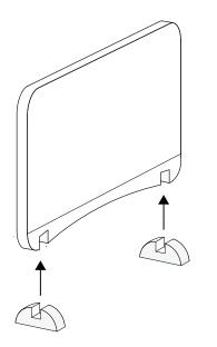
Step 1 Remove divider and support leg (x2) from box
