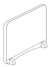
**Step 2** Push legs in place till flush with bottom of screen
